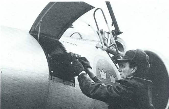
Maintenance technician removes faulty LRU. Almost 25% of Viggen skin is covered by hatches to simplify equipment accessibility. LRUs are field-replaceable without adjustment.
