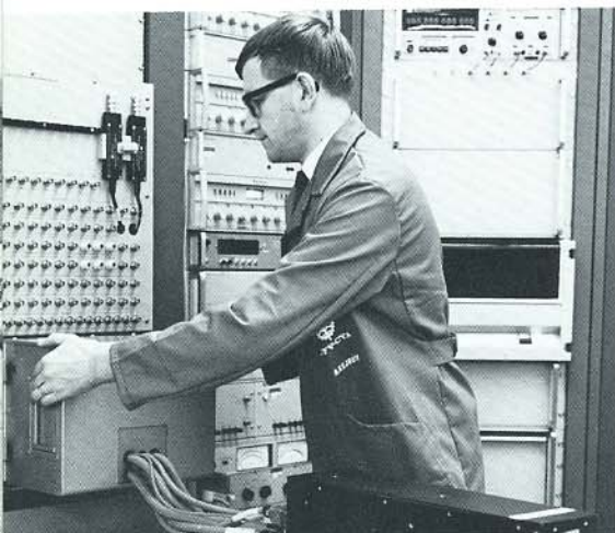
Technician plugs LRU test adapter into interface panel on B-level test system.
